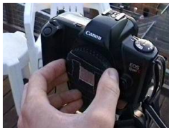
Figure: Remove camera lens
